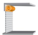
New: The EFA-SST® PS features a spiral construction that significantly reduces the space requirements in the lintel.
