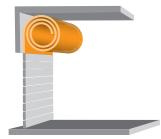
The round spiral is the standard and best solution when you have ample space above the door.
